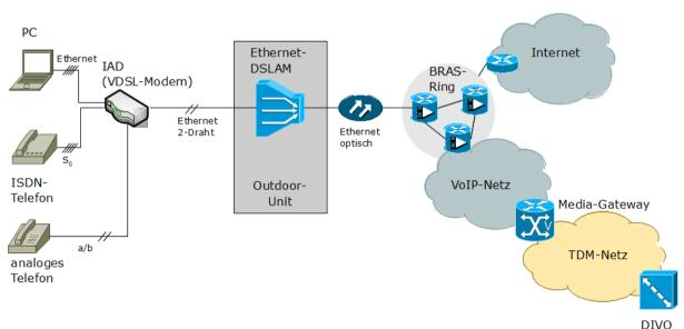
IAD: integrated access device (DSL-Modem, Router, Switch, WLAN-AP,...)
